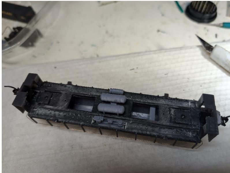
Note that the small airtank has a flat end, this end faces the "B" end of the frame. The three air brake components on the other side have a detent in the frame to align the parts with. The control valve (with squarish item on one end) goes toward the "B" end.
